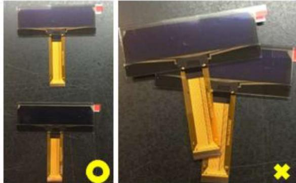
5. Avoid jerk and excessive bend on TAB/FPC/COF, and be careful not to let foreign matter or bezel damage the film.
