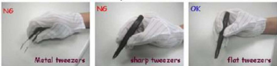
8. Please do not bend the film near the substrate glass. It could cause film peeling and TAB/FPC/COF damage. For TAB, It should bend the slit area as actual OLED it is. For FPC or COF, it is suggested to follow below pictures for instruction (distance between substrate glass and bending area >1.5mm; R>0.5mm).
