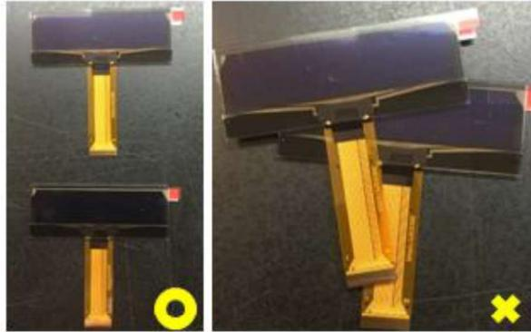
5. Avoid jerk and excessive bend on TAB/FPC/COF, and be careful not to let foreign matter or bezel damage the film.
