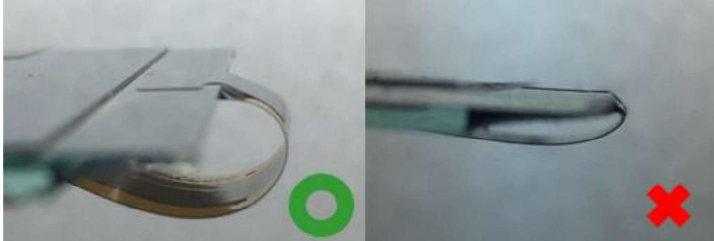
9. Avoid bending the film at IC bonding area. It could damage the IC ILB bonding. It should avoid bending the IC seal area. Please keep the bending distance >1.5mm.
